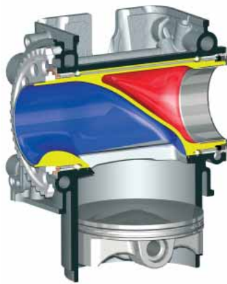
Figure 6: Section through Rotary Valve Cylinder Head Assembly.
